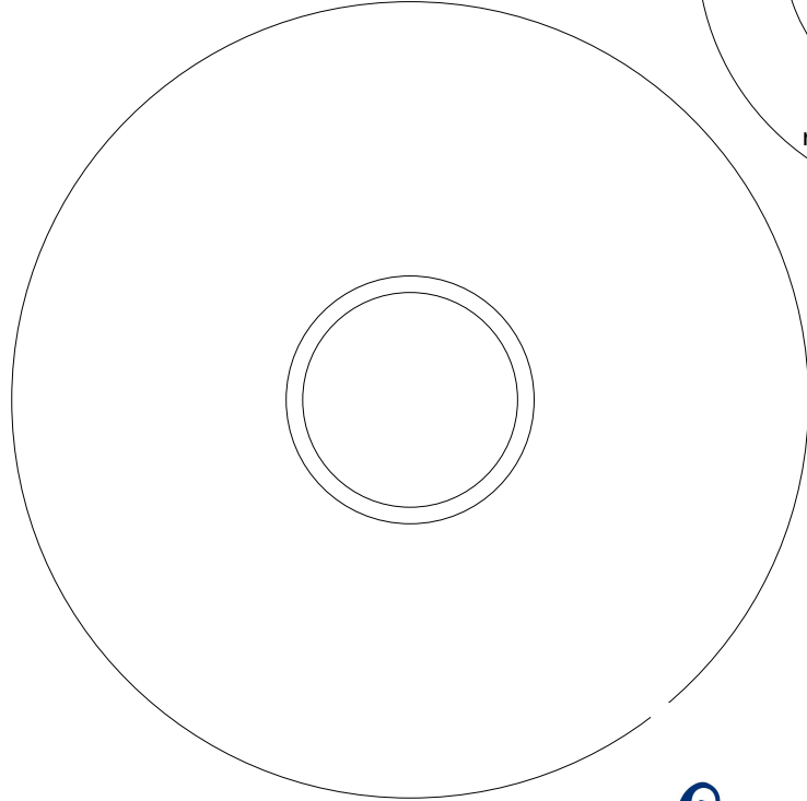
24mm motor mount centering rings with 29mm option
